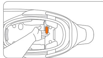
2. Open the driver's footrest, which is also the battery compartment lid, and take out the battery.
