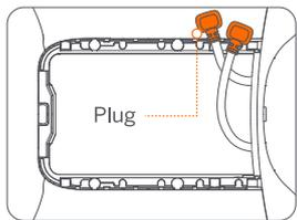
**NOTE:** Before installation, make sure there are no foreign objects in the battery compartment with two plugs inside.
