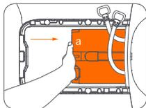
3. Connect the battery plug on the corresponding side.
