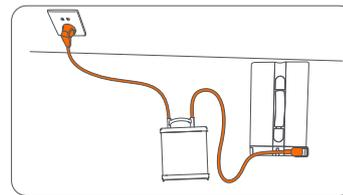
\* The indicator on the battery charger shows solid red when charging and turns green when finished.
