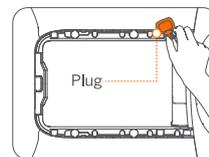
**NOTE:** Before installation, make sure there is no foreign object in the battery compartment and there is only one plug inside.
