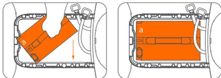
2. Push the battery (a) to the inner end.
