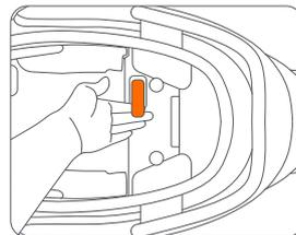
a. Open the seat bucket with your key, and pull the foot panel switch to unlock it.
